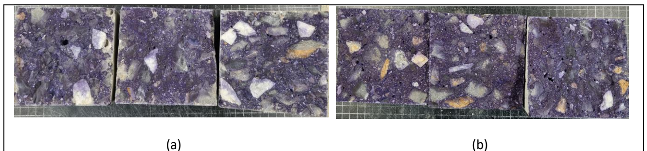
Figure A. 10: Accelerated carbonation of (a) three CEM II/A-V (Ref.) and (b) three CEM IV/A (V) samples after 28 days of testing
